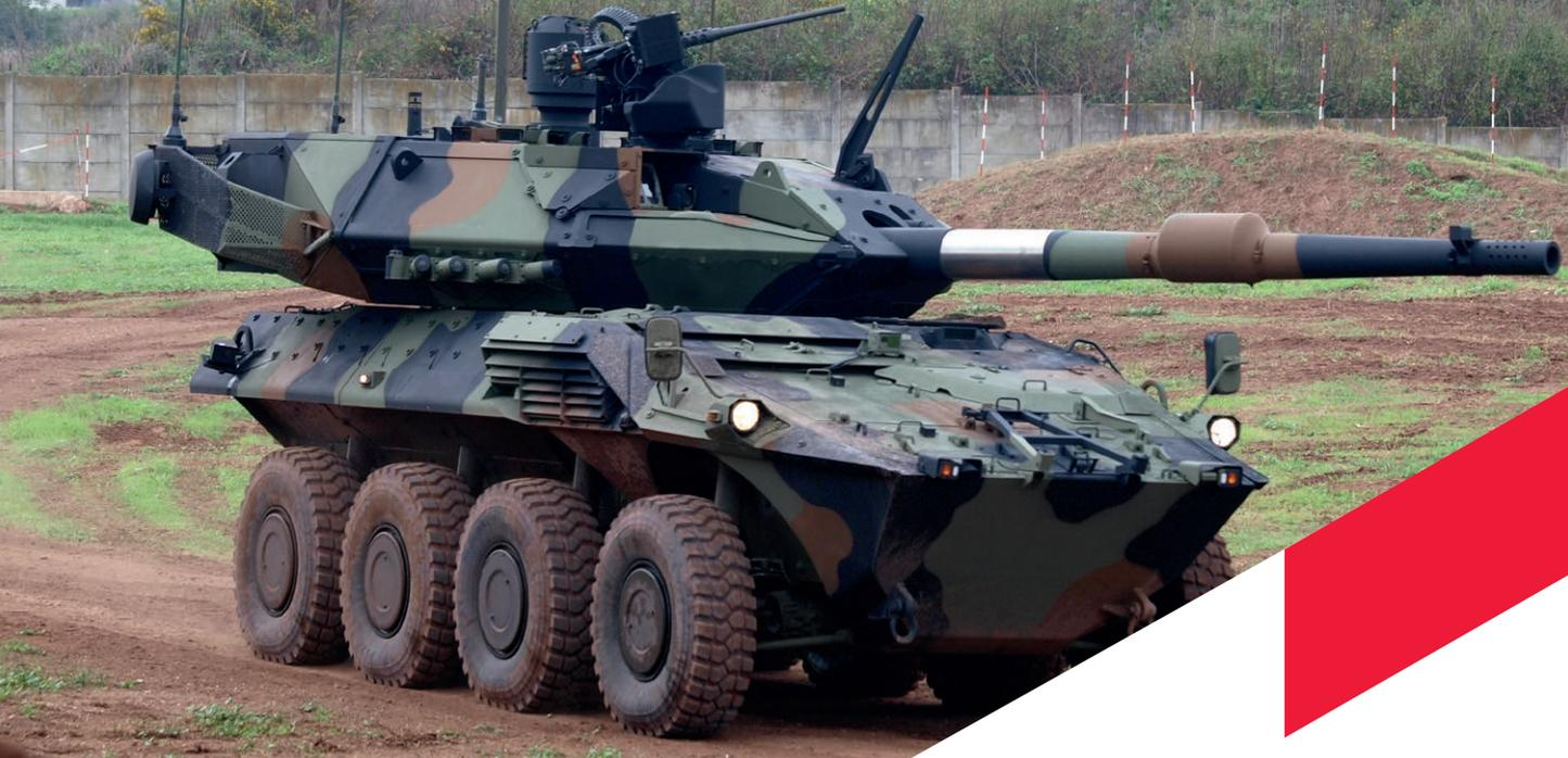
The HITFACT® MkII represents a new stage in the evolution of the combat proven HITFACT® family, the first Large Caliber Turret in the world equipped with an high pressure MBT gun installed on a 8x8 wheeled vehicle, exceeding the 500 units in service with several Armies.
