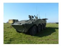
The **Centauro VBM Mortar Carrier** shares the characteristics of mobility and versatility typical of the Centauro family. Its platform is fitted with a 120 mm rifled mortar that offers many advantages in terms of precision, range, operativeness and ergonomy thanks to its semi-automatic loading system.
