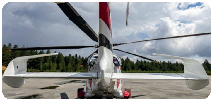
Figure 10 - Installed ORIGAMI winglet for flight test activity
