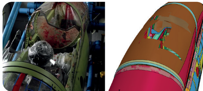
Figure 2-M345 Blastshield FEM Experimental Test correlation
