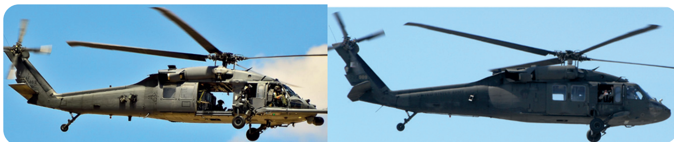
Figure 3 - UH-60 tiltable tailplane solution: high-speed position (left) vs low-speed position (right)
