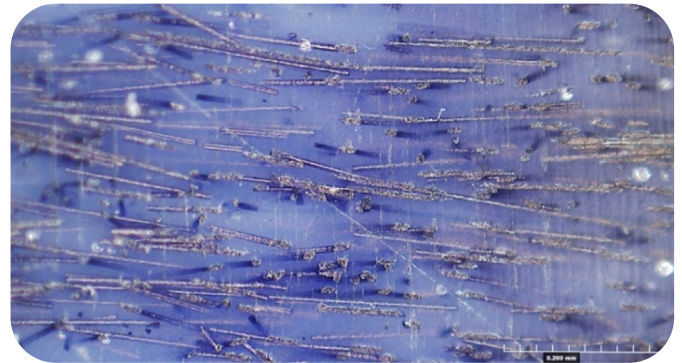
8-OM images of fibres in 90deg specimens in the longitudinal section with respect to the direction of filament deposition
